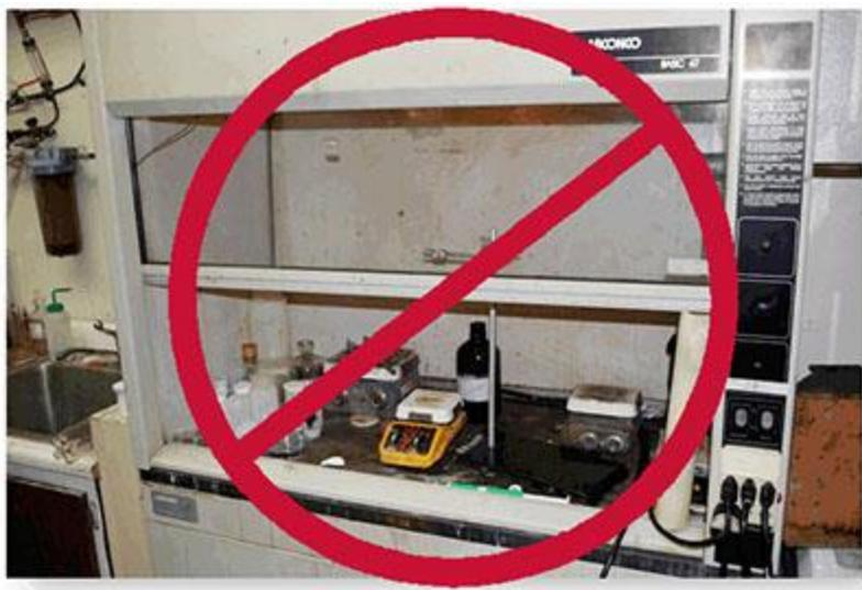
Do not use your fume hood as a storage cabinet. From labs I have seen, this is the biggest offender. Doing so can lead to accidental spills of a large concentration of chemicals. When chemicals are not in use, be sure to store them in cabinets appropriate for the chemical.
