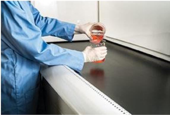
Operate at least 6 inches inside the fume hood behind the plane of the sash. This is important for safety as a good working practice, stated by industry standards such as ANSI/AIHA Z9.5. This means that any equipment placed in the fume hood should not be touching the airfoil along the front of the work surface.
